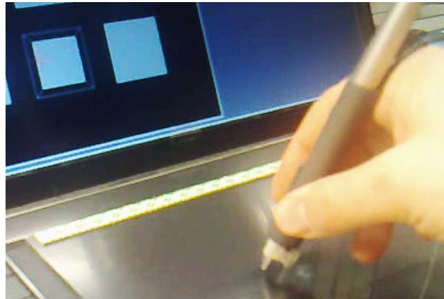
figure 3. User testing the illusion with 3D-Press augmented with a visual representation. While the user already perceives haptically that the rigid plastic surface is actually compliant when pressed with the augmented stylus, a visualization of the same model can reinforce and even model the illusion
